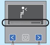
It is possible to vary the jet pair activation speed. Press the "<" key to decrease or the ">" key to increase the speed.
