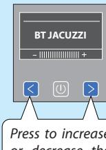
Press to increase or decrease the volume. Subsequent to connection of the Bluetooth® device, the display will show the following configuration.
