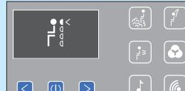
When the keys are pressed, an arrow appears. Move the arrow to the pair which is to be disabled.
