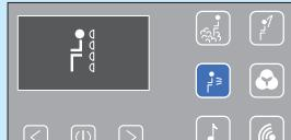
The jet pairs are activated (represented by 4 half-circles) from the bottom upward in sequence. Each pair remains active for 3 seconds.
