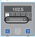
Press to increase or decrease the volume. Keep the "<" key pressed down to mute the sound. To restore the sound, press the "<" or ">" keys.
