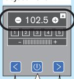
1 Press to tune in the first frequency with a strong signal. The automatic search will be disabled when kept pressed down for a few seconds.
