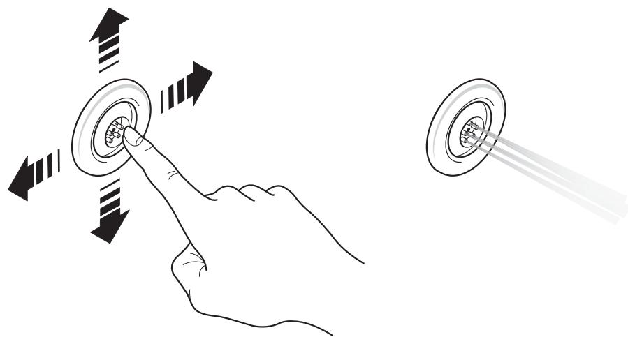
*Each jet can be tilted by pressing the nozzle and moving it in the desired direction.*
