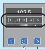
1 Press. 2 Press "<" or ">" to select the position where the selected frequency should be stored (the position is shown by a broken outline).
