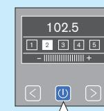
Keep pressed down for a few seconds. The selected position will be displayed with a white background and a double acoustic signal will sound, indicating that it has been stored.
